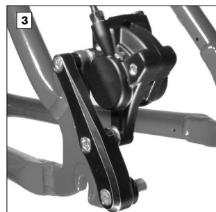
Mounted Rohloff SPEEDBONE, view from outside the frame.
