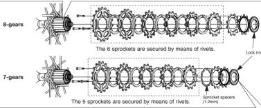
For installation of the HG sprockets, use the special tool (TL-LR15) to tighten the lock ring.
