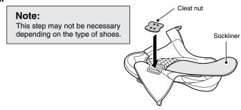
**3.** From the bottom of the shoe, position a cleat and then a cleat adapter over the cleat holes. The cleats are compatible with both left and right pedals. Provisionally tighten the cleat mounting bolts.
