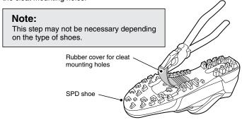
**2.** Remove the sockliner and position a cleat nut over the oval holes.
