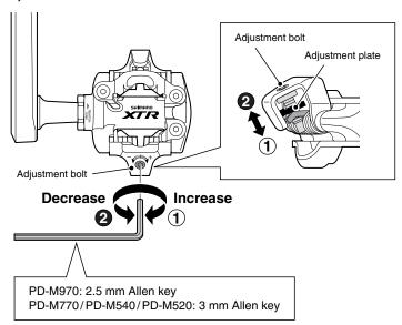
When the adjustment bolt is turned clockwise, the spring tension increases, and when it is turned counterclockwise, the spring tension decreases.
