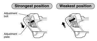
If the adjustment plate is at the strongest or the weakest position, do not turn the adjustment bolt any further.
