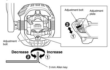
When the adjustment bolt is turned clockwise, the spring tension increases, and when it is turned counterclockwise, the spring tension decreases.
