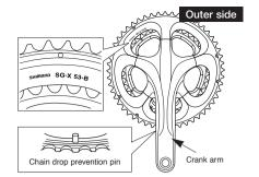
With the marked surface of the smaller chainring facing away from the crank arm, set the chainring so that the \( \widehight) mark is lined up with the crank arm position.
