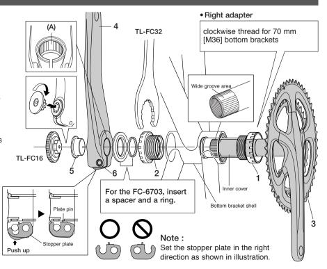
Push in the stopper plate and check that the plate pin is
