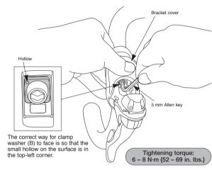
When installing the components to carbon frame/handle bar surfaces, verify with the manufacturer of the carbon frame/parts for their recommendation on tightening torque in order to prevent over tightening that can cause damage to the carbon material and/or under tightening that can cause lack of fixing strength for the components.
