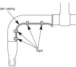
Then wrap the handlebar with handlebar tape
